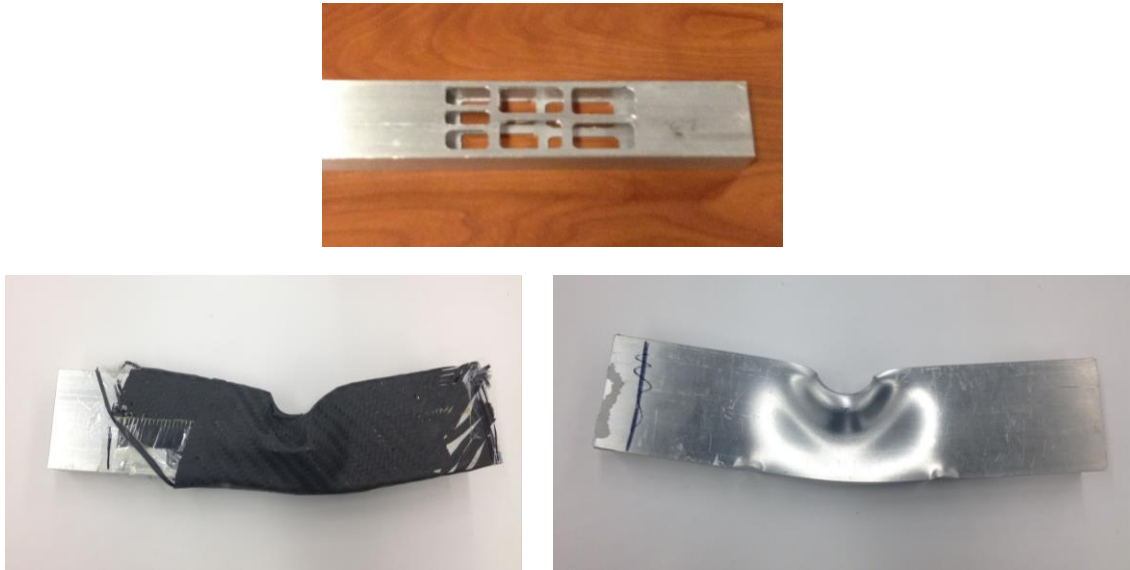
Figure 17: Aluminum tubing carbon fiber reinforcement test pieces.
