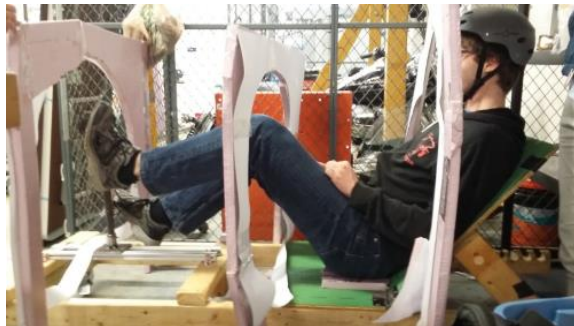
Figure 16: Fairing fit verification setup.
