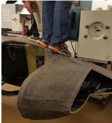
Figure 14: RPS side load test setup.
