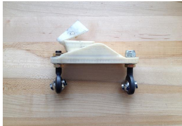
Figure 20: 3D printed steering knuckle with failure along nylon-fiber boundary layer.
