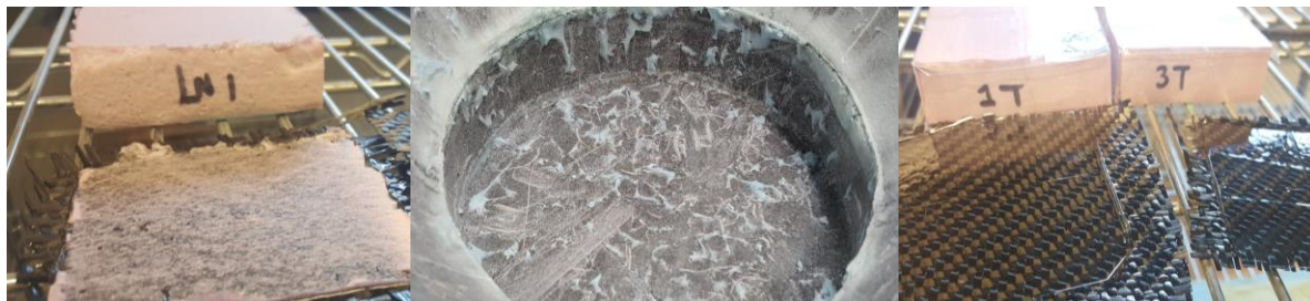
Figure 21: Mold release testing (no epoxy, rubbing compound, tape).
