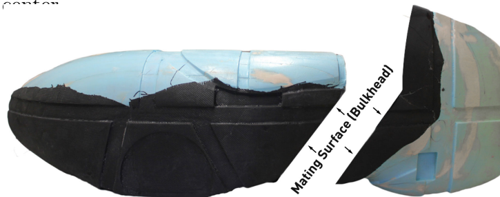
Figure 1: Two male mold halves before joining.
