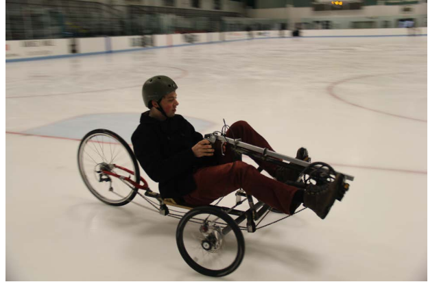
Figure 2: On ice, the vehicle was completely stable during tight turns and slides.
