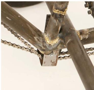
*Figure 24: Fully-contained chain idlers keep the chain on the pulleys.*
