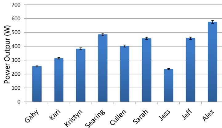
Figure 31: Average power output over 15 seconds for 9 team members. The error bars were determined by assuming perfectly precise electrical power measurements, and propagating the standard errors of the mechanical power regression into the power equation.
