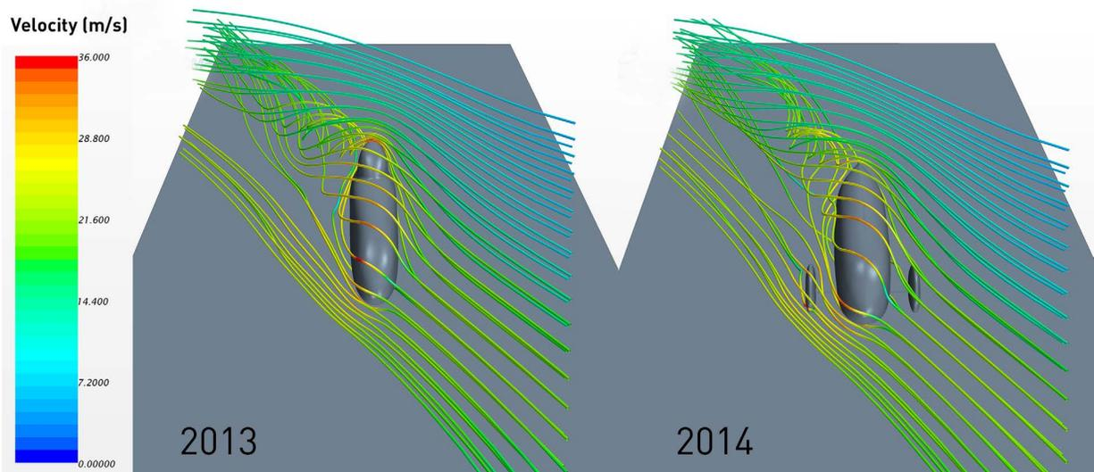
*Figure 15: The crosswind flow profiles demonstrate Cheryl's improved crosswind aerodynamics. Note the decrease in major flow disturbances around Cheryl compared to The Plaid Panther.*
