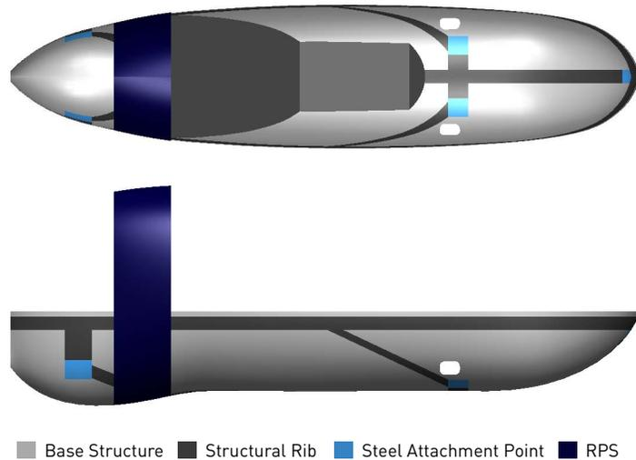
Figure 2: Monocoque Structural Rib Configuration
