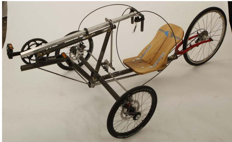
*Figure 23: Tadpole Tricycle Prototype*
