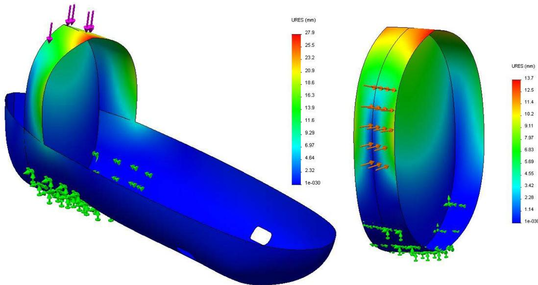
Figure 9: Simulated displacement of the rollover protection system when subjected to a 600lb top load at 12° from vertical (left) and a 300lb side load at shoulder level (right).
