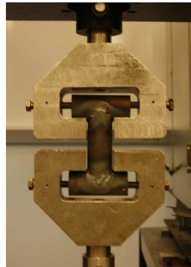
Figure 33: Steel tube connection test setup.
