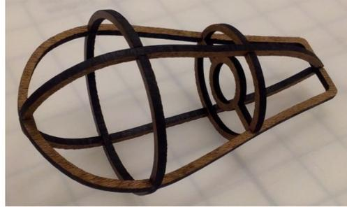
Figure 27: Ribbed test specimen for wind tunnel testing.
