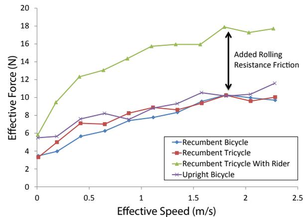
Figure 32: Friction measurements for various vehicles
