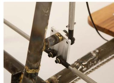
Figure 5: Steering Linkage Intermediate Link
