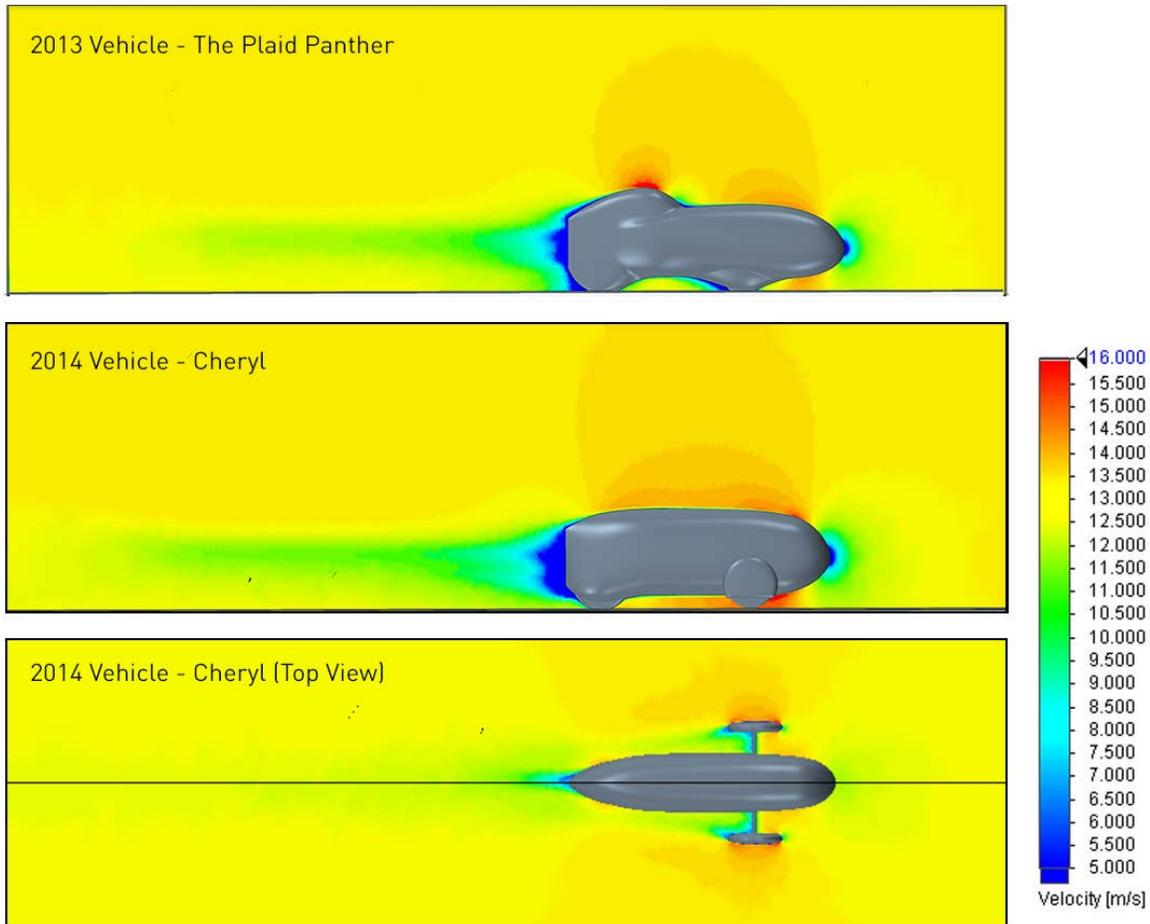
*Figure 14: Simulated fluid velocity profiles for Cheryl and The Plaid Panther. Note the increased stagnation regions behind Cheryl's wheels and tail.*
