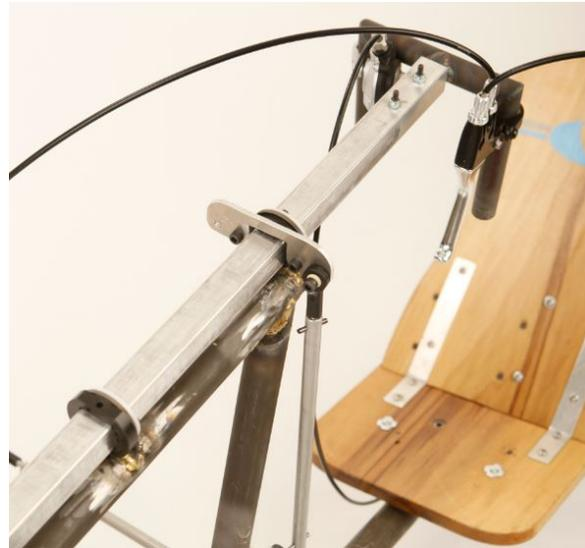
Figure 4: Telescoping Handlebar Linkage
