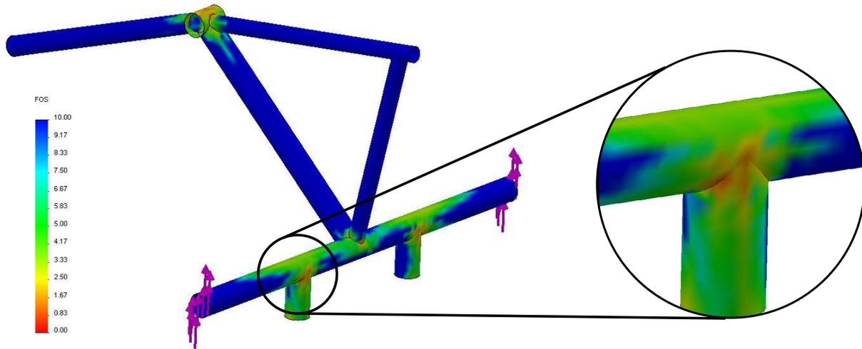
Figure 10: Front frame finite element analysis results. Note the low factor of safety at the rear monocoque connection points.
