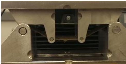
Figure 25: Four point bend testing was performed on all candidate fabrics.
