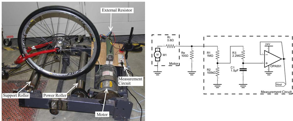
Figure 30: The dynamometer apparatus. Left: The dynamometer electrical system. Right: a picture of the dynamometer with the tricycle.
