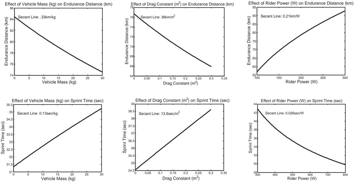
Figure 18: Summary of simulation results. Each plot shows the effect of various design parameters on endurance distance or sprint time. Secant lines give the average slope over the plot area.
