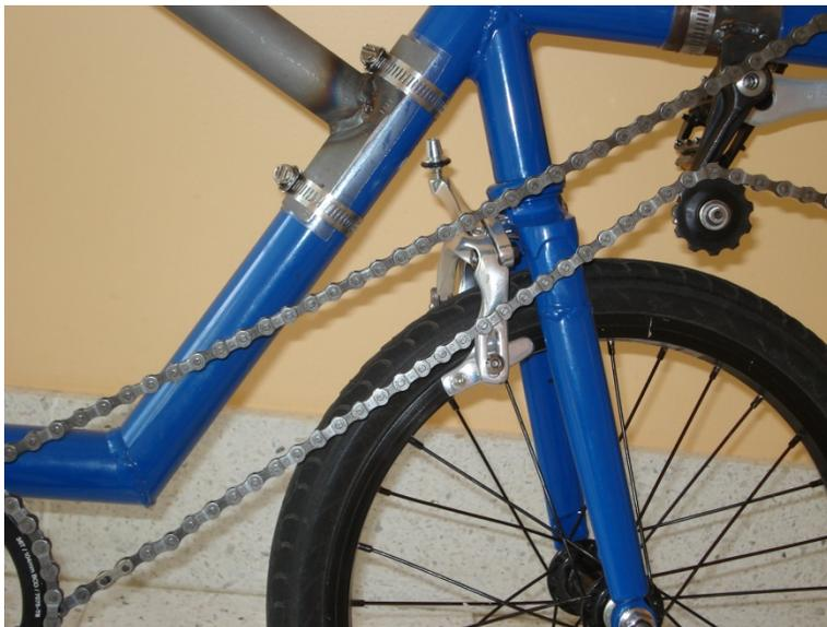
**FIGURE 1: THE PROXIMITY OF THE CHAIN PATH TO THE BRAKES AND FRONT FORK NECESSITATES MOUNTING BRAKES BACKWARDS BECAUSE OF INTERFERENCE ISSUES.**
