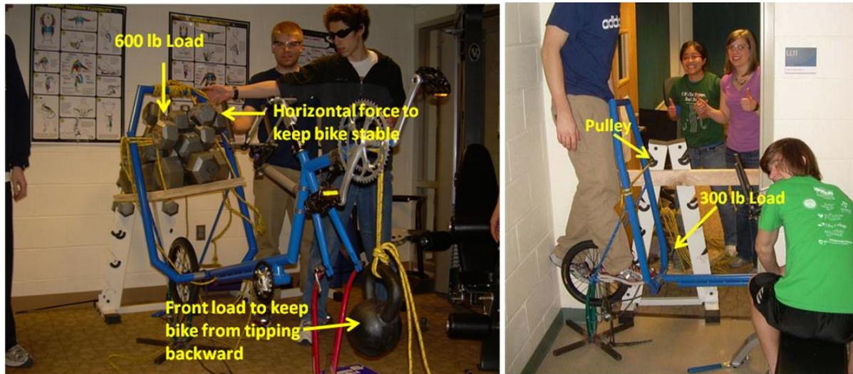
FIGURE 19: LEFT IS THE ROLL BAR SUCCESSFULLY WITHSTANDING 600LB LOAD AT 12° FROM VERTICAL. RIGHT SHOWS ROLL BAR UNDER 300LB SIDE LOAD. TEAM MEMBERS STANDING ON REAR FORK AND SEATED IN FOREGROUND ARE PROVIDING REACTION FORCES TO COUNTER THE MOMENT APPLIED BY THE LOAD.
