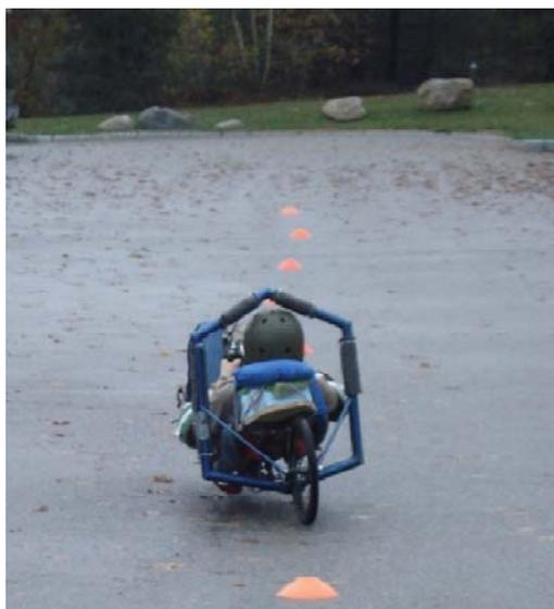
FIGURE 17: THE FEMALE RIDER MANEUVERING THROUGH THE CONES ON THE VEGA FOR THE STABILITY AND HANDLING TEST.
