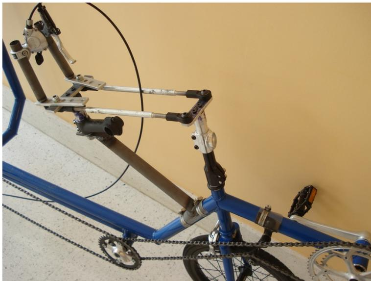
FIGURE 2: STEERING SYSTEM OF *HELIOS*, SHOWING DOUBLE PUSHROD SETUP WITH ADJUSTABLE LENGTH HANDLEBARS IN UPPER LEFT.
