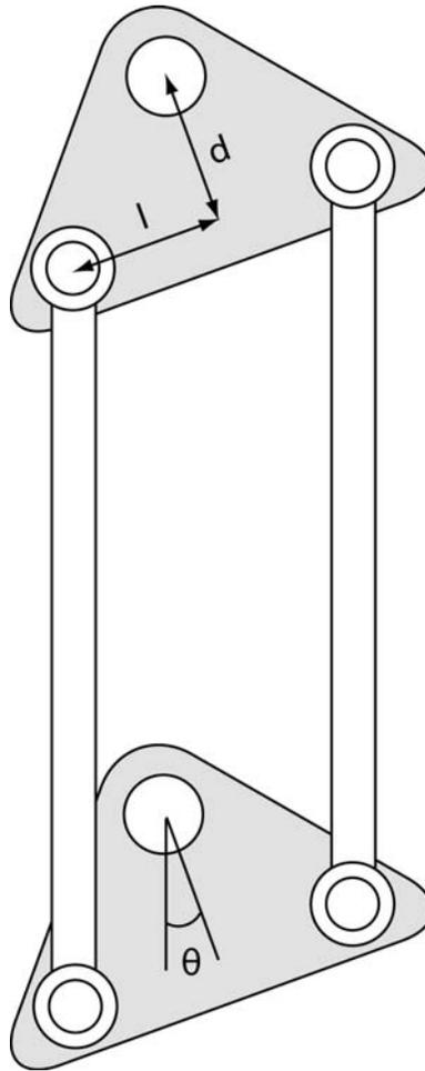
**Figure 11.** Diagram of offset steering geometry.
