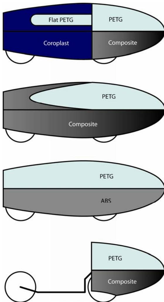
**Figure 3.** Fairing construction options.
