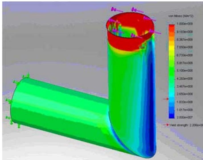
**Figure 6.** Miter joint with plate.
