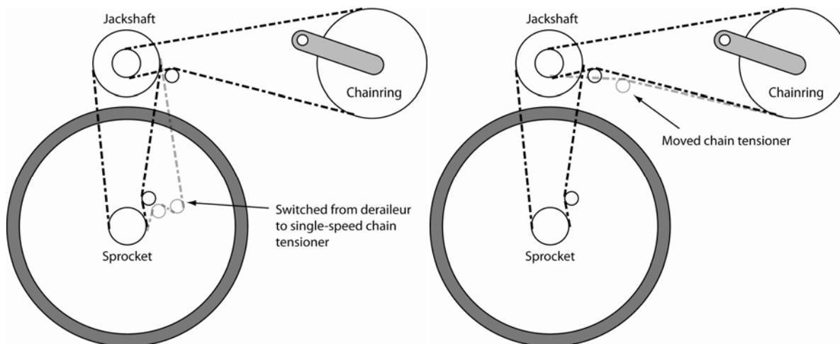
**Figure 2.** Chain line improvements: black path shows improvements over last year's chain path, shown in gray.
