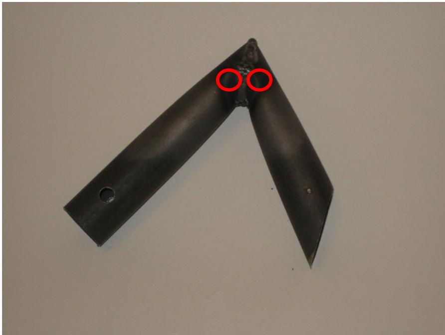
**Figure 19.** Photograph of miter joint with plate after testing. The buckling points appear to be more even.
