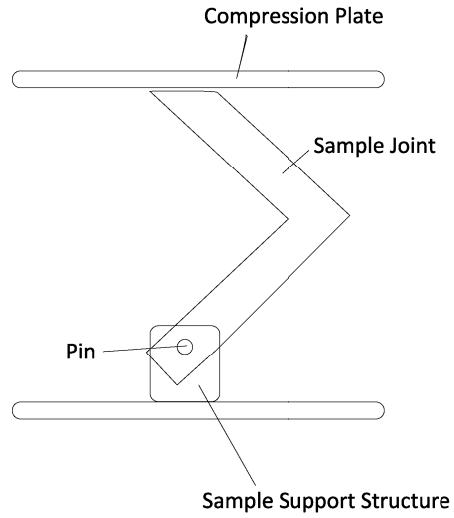
**Figure 15.** Compression Test Setup.
