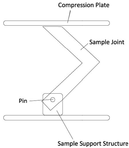
**Figure 15.** Compression Test Setup.
