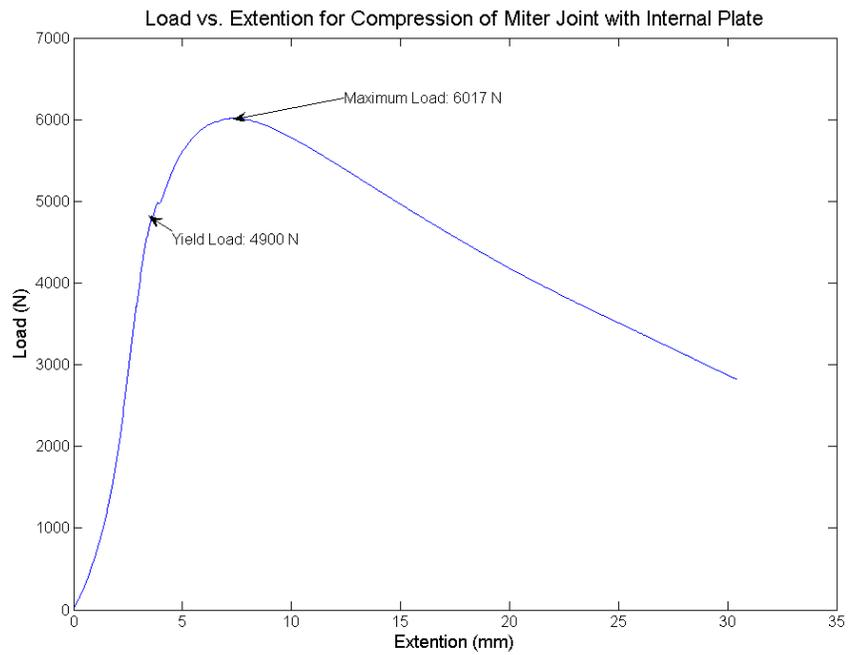
**Figure 18.** Load extension graph for the miter joint with an internal plate. Yield load is at 4900 N and maximum load is at 6017 N.
