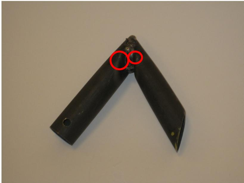
**Figure 17.** Photograph of open miter joint after testing. The two buckling points are circled in red.
