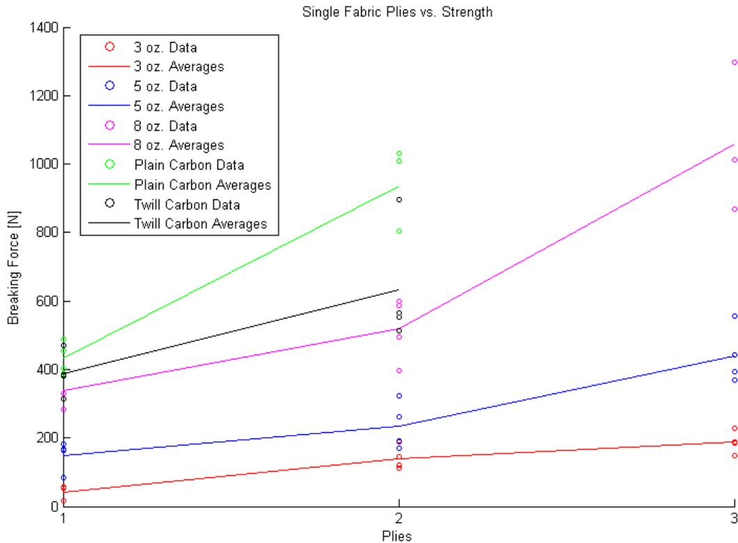
**Figure 23.** There is clearly a correlation between number of plies and strength of the resulting article. However, it does not seem like this correlation is always of the form *single ply strength × number of plies = strength*.
