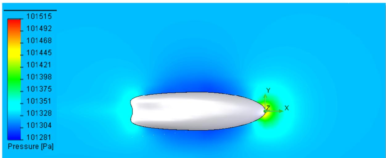
**Figure 10.** Pressure gradient for modified airfoil design. Maximum Pressure: 101697Pa.
