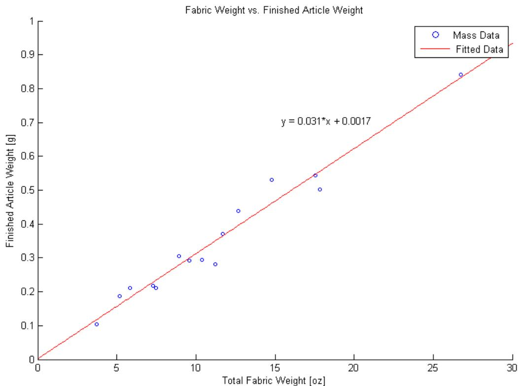
**Figure 24.** This figure shows the relationship between cumulative fabric weight and finished article weight. Cumulative fabric weight was found by adding the weight (in oz) of all the cloth used in the piece, while the finished article weight was found by simply massing the article on a scale.
