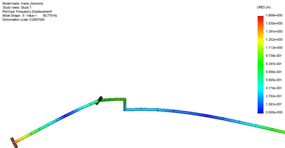
**Figure 13.** Mode shape for fundamental excitation frequency of 90 Hz. The flexing is out of plane of the frame.
