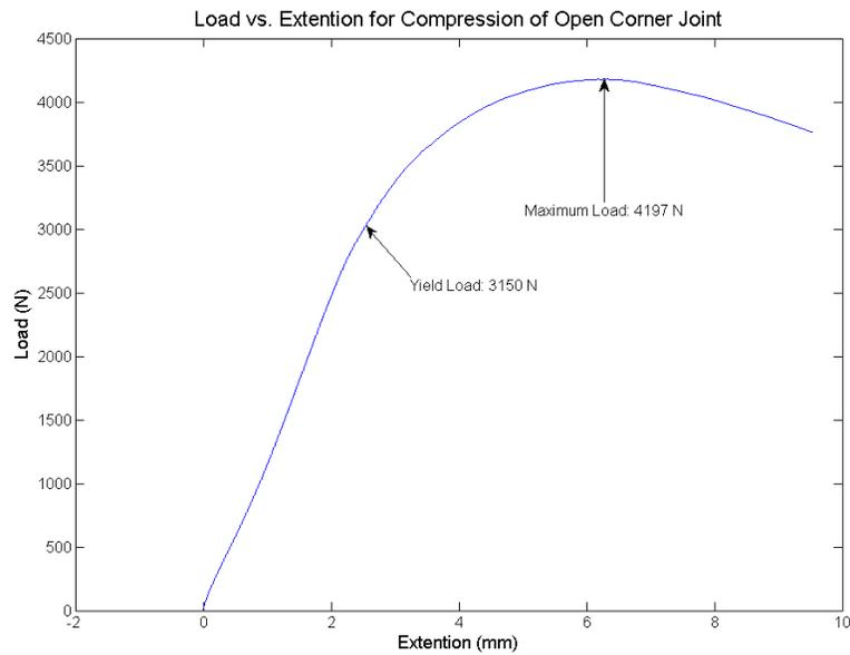
**Figure 20.** Load extension graph for the open corner joint. Yield load is at 3150 N and maximum load is at 4197 N.
