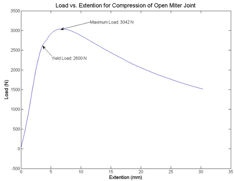
**Figure 16.** Load extension graph for the open miter joint. Yield load is at 2600 N and maximum load is at 3042 N.
