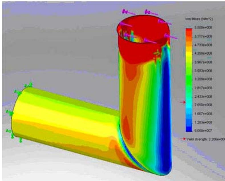
**Figure 7.** Side view of plated miter joint.
