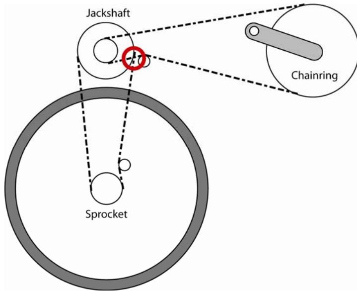
**Figure 1.** Red circle indicates region of chain interference.
