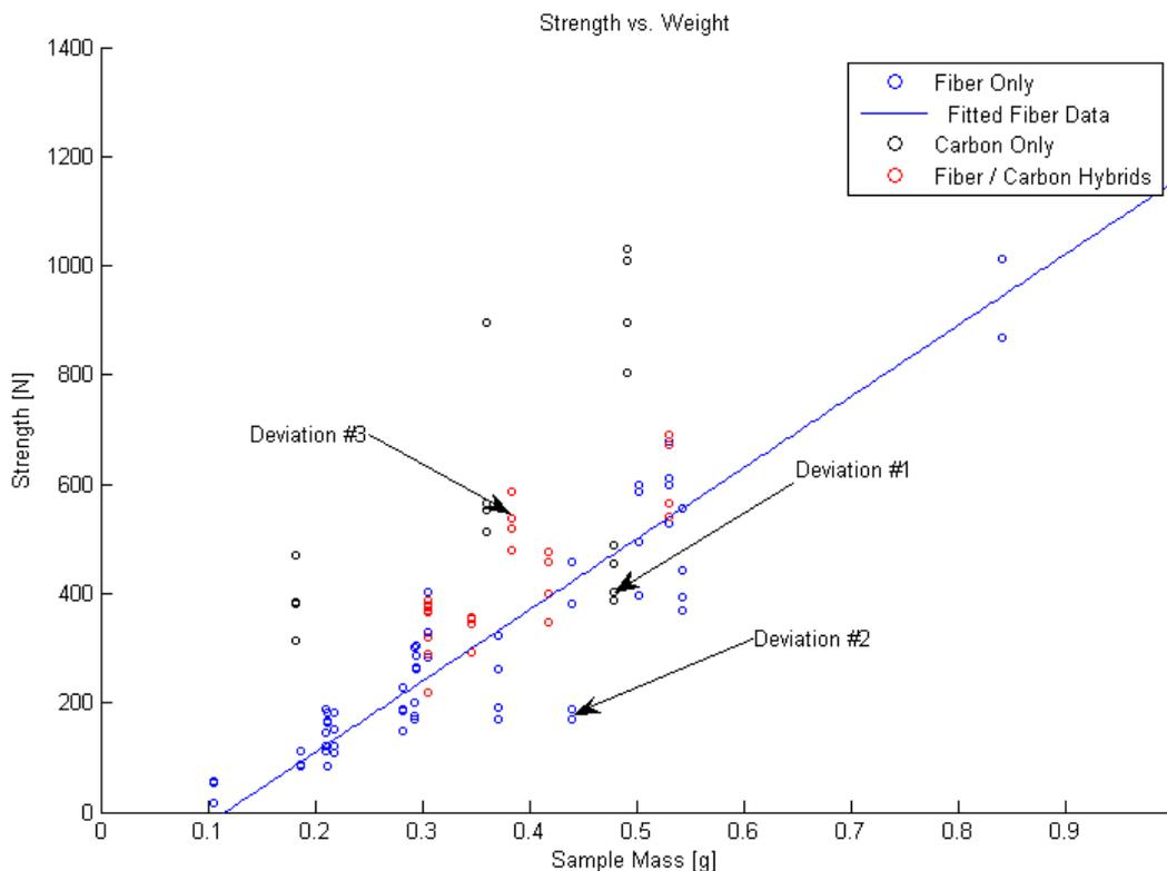
**Figure 25.** Note that many sample sets had one or even two significant outliers, probably caused by manufacturing defects or weave directionality.
