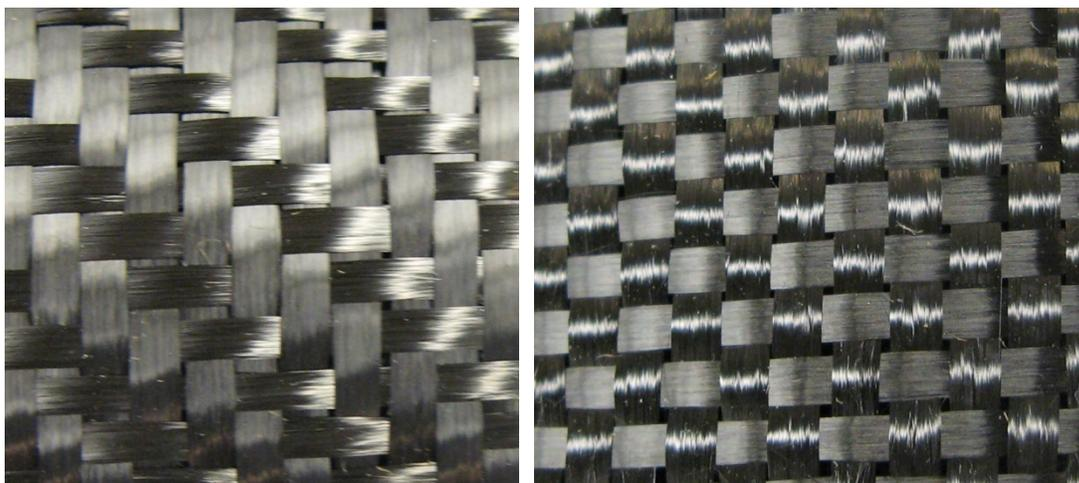
**Figure 22.** The above image shows a visual comparison between the two main types of carbon fiber weave. On the left is a plain weave (directional) while on the right is a twill weave (non-directional).
