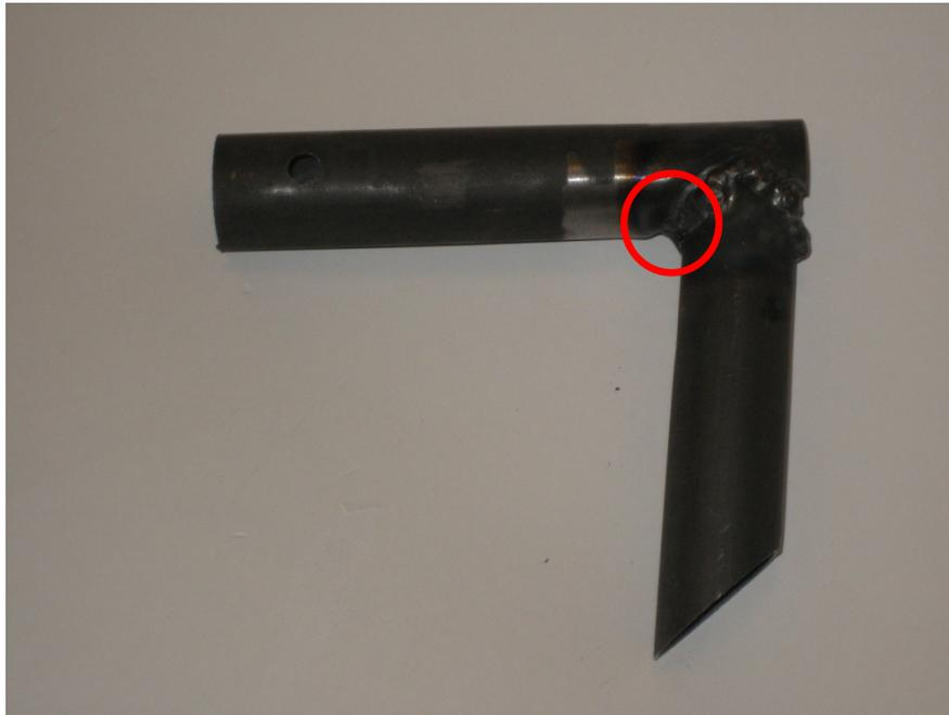
**Figure 21.** Photograph of the open corner joint after testing, with the buckling point circled in red.
