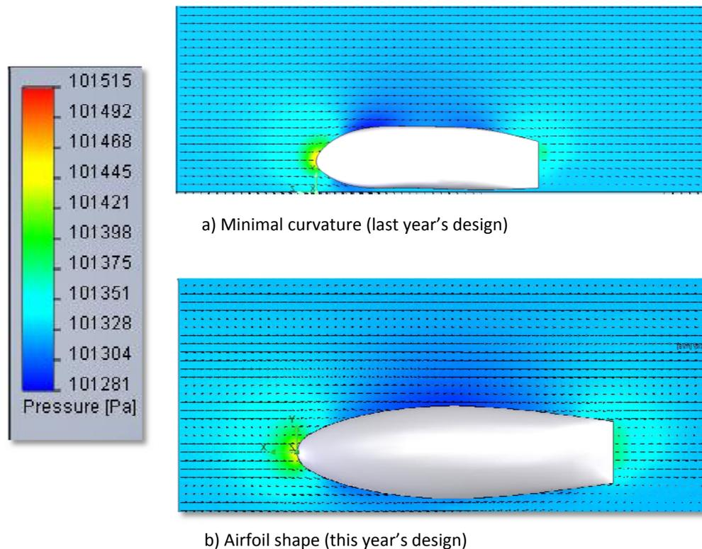
**Figure 9.** Pressure gradients for fairing designs: a) Minimal curvature (Maximum Pressure: 101515Pa); b) Airfoil shape (Maximum Pressure: 101554Pa)
