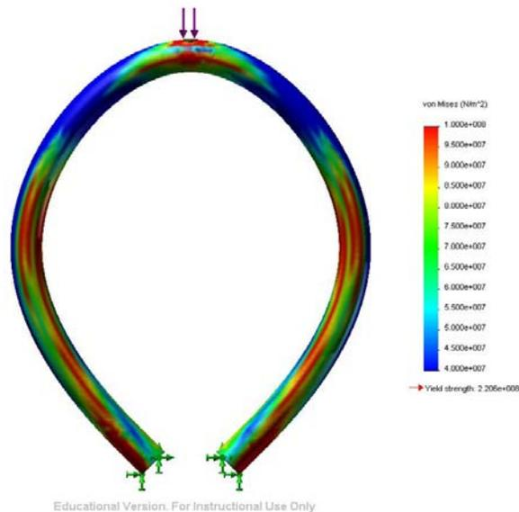
**Figure 14.** COSMOSWorks output for loading of roll bar.
