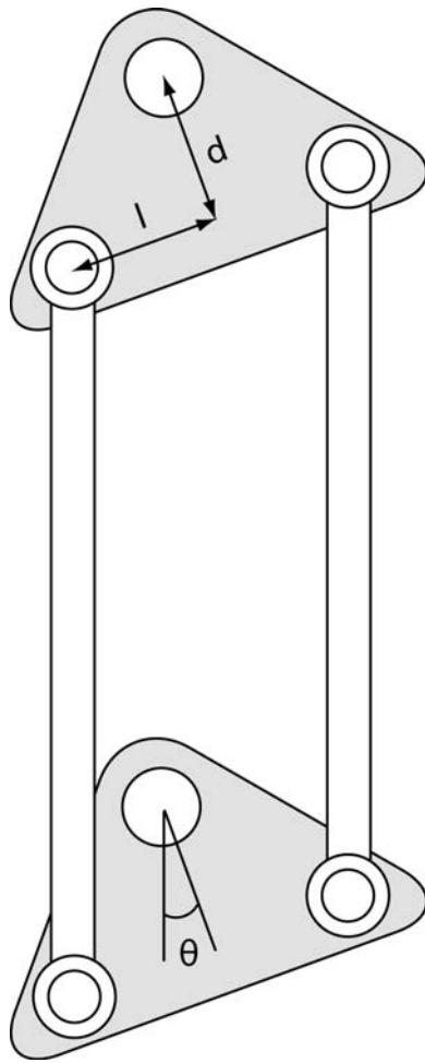
**Figure 11.** Diagram of offset steering geometry.
