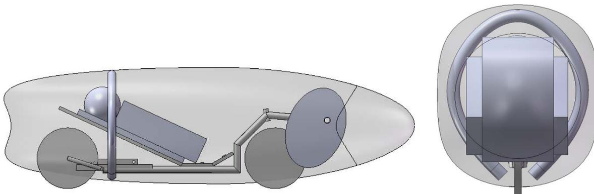
**Figure 26.** The roll bar is placed at the head of the rider and surrounds the shoulders as well as the pedal path.
