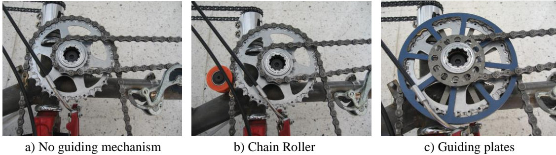
Figure 2: Various methods of guiding chain through the jackshaft.
