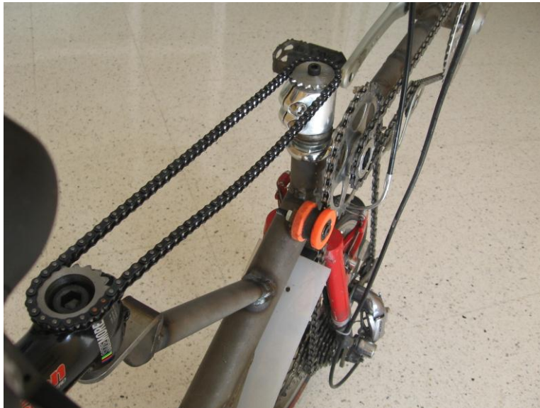
Figure 7: Chain steering mechanism showing slack while turning.
