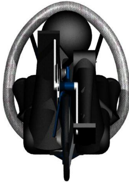
Figure 24: The roll bar is designed to fully surround the rider so that it would be the first to hit in any impact situation.
